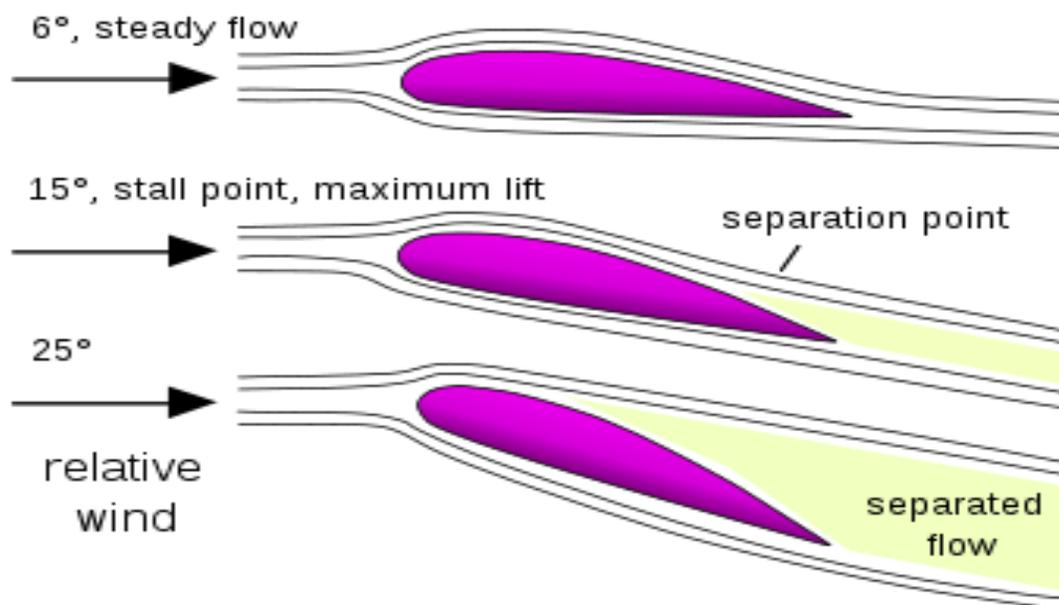
A fixed-wing aircraft can stall in any pitch attitude or bank angle at any airspeed but commonly occurs while reducing the speed to the un-accelerated stall speed. Un-
