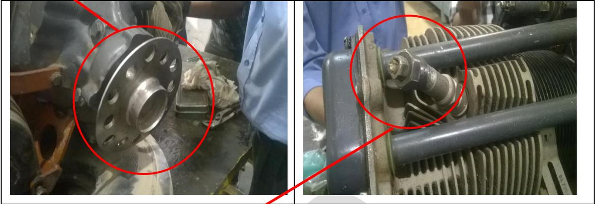
4. Cylinder No. 02 top spark plug harness broken from magneto side
