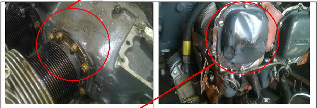
2. Cylinder No. 2 rocker box damaged.
