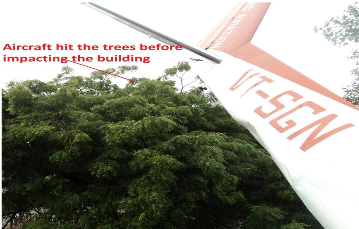
Thereafter the aircraft main wheel rolled on the building top and the aircraft got air borne again. While executing a 180 degree turn it hit a tall tree next to the building as it was evident from the dent/impact marks observed on the fuselage / wing structure and also the marks on the tree top.
