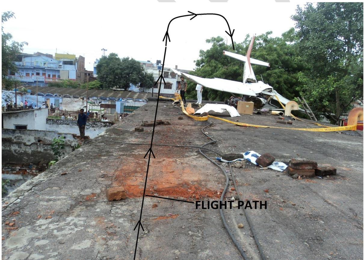
***Flight path of the aircraft before impacting the building***
